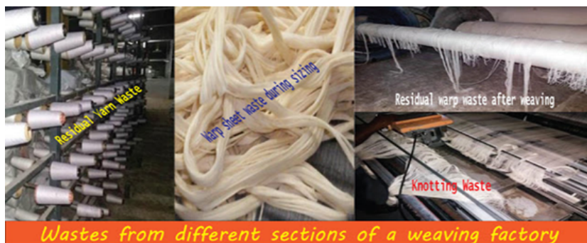
Figure 31: bottoms, Size waste, residual warp waste after weaving. Knitting waste recycled
