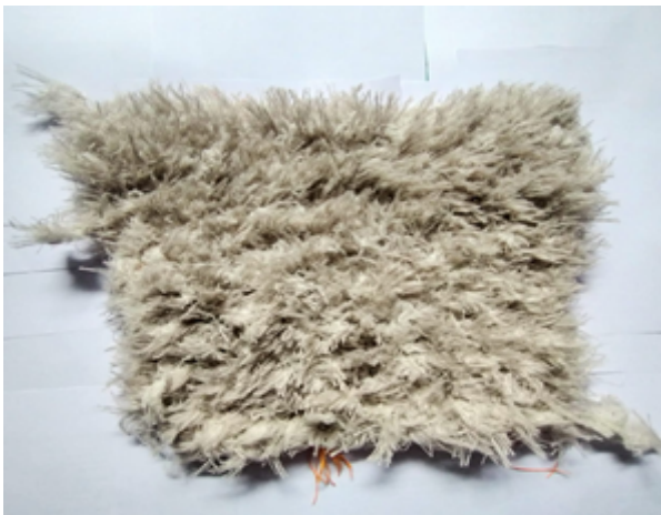
Figure 26: Matt Produced from the Auxiliary Selvage
