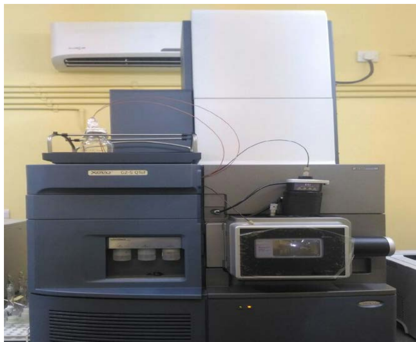
Figure 13: Instrumental Setup of High-Resolution Mass Spectrometry (HRMS) - Waters XEVO G2-S QTOF System
