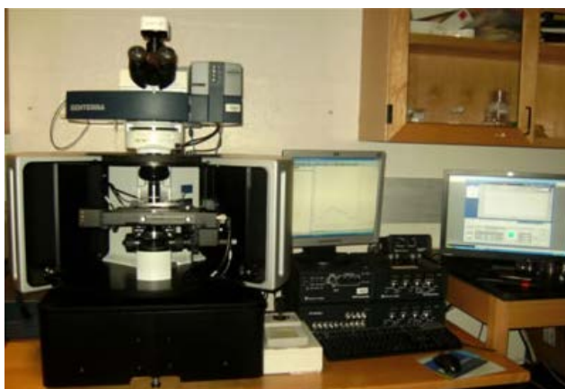
Figure 10: Instrumental Setup of Atomic Force microscopy (AFM), 2010 NT-MDT NOVA-1.0.26
