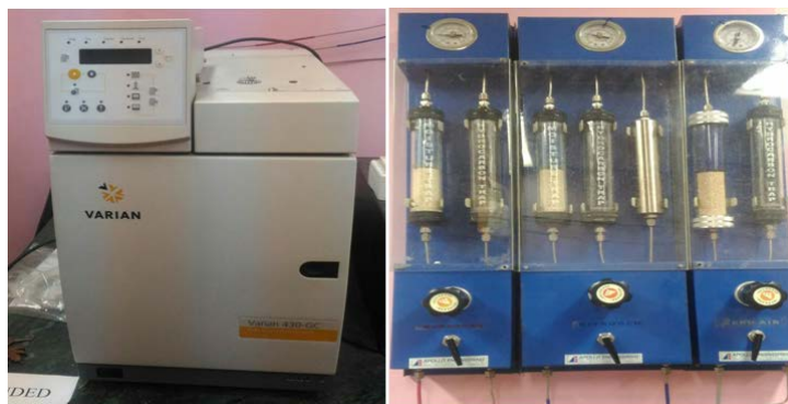
Figure 14: Instrumental Setup of Gas Chromatography (GC)- Varian 430, 30m CP-SIL8CB Capillary Column System
