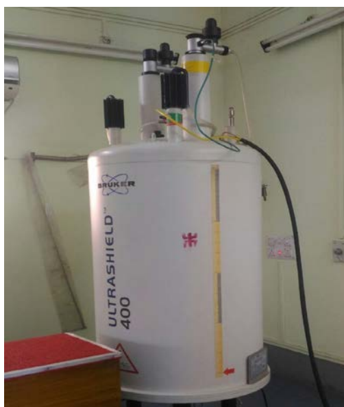
Figure 11: Instrumental Setup of Nuclear Magnetic Resonance (NMR) - Bruker Ultrashield 400 MHz Spectrometer Used in the Present Work.
